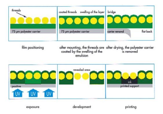
Its use is simple, quick and clean. The film is mounted by capillarity after wetting both sides of the screen.
