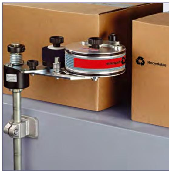
These devices are available in 1 marking circumference : 430 mm. 3 marking heights : 25, 50 and 100 mm.
