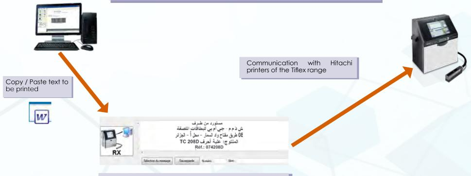
Interface allows visualisation and modification of position of the text for marking (number of lines, font size, page layout...)
